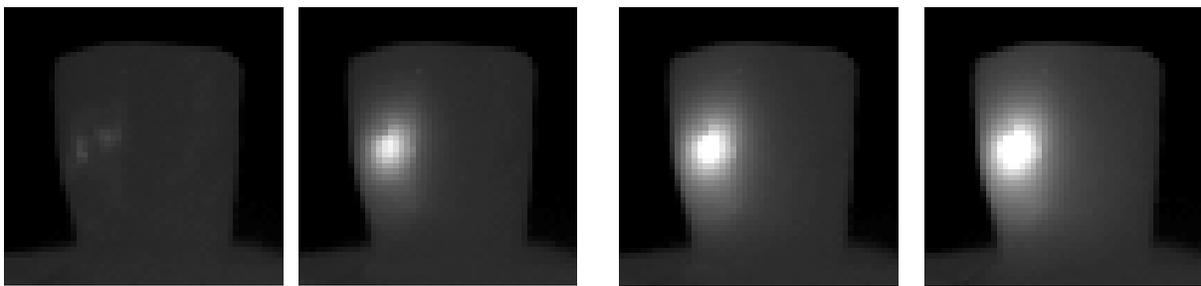
Figure 19 - Thermal images from the infrared camera reported in grey scale, relative to the laser exposure, after 0.16 s, 1.6 s, 3.2 s and 4.8 s.
