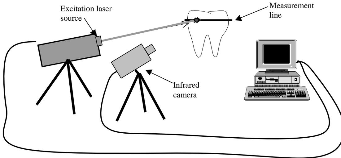
Figure 1 - Schematic of the experimental arrangement.
